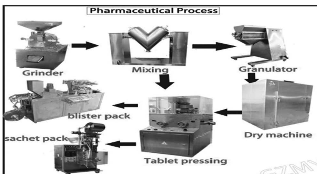
FIGURE 6.3 A typical conventional batch manufacturing process for tablets.
